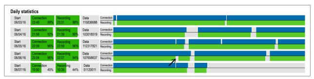
Figure 3 – PoIP provides daily statistics of connection (blue line) and recoding (green line) data of signal transmission in the server. It is of note that connection and transmission percentages are very similar to each other (day 3/6: 99% and 98%, day 4/6: 92% and 90%, day 5/6: 96% and 96%). Small losses occurred, as on 6/6/2016, when there was a brief period when signal was transmitted but not recorded in the server (arrow)
