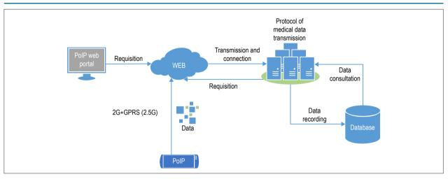
Figure 1 – Conceptual diagram of PoIP – as can be seen in the diagram, PoIP uses the concept of real-time transmission of the data by the EDGE technology. Wireless data transmission is performed by standard protocol to internet access in mobile devices by GPRS-EDGE – Generic Packet Radio Service, commonly known as 2.5G
